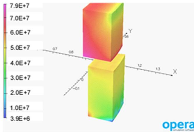
Fig. 4. Hoop stress [Pa] in the winding, mode A.
