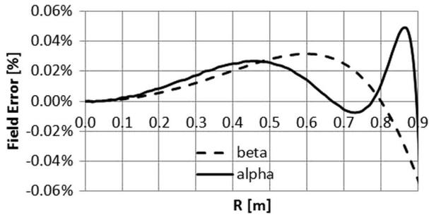
Fig. 1. Field deviations from the old form factors in alpha coil and beta coil versus radius.
