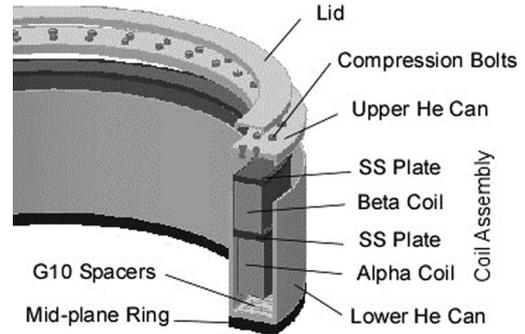
Fig. 3. Cold mass parts illustrating assembly sequence.
