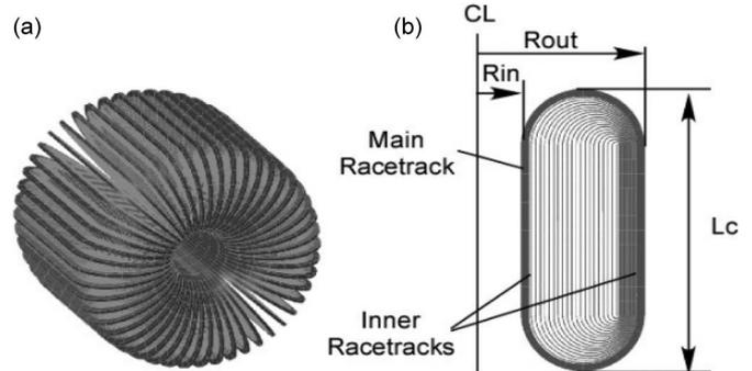
Fig. 1. CTF: (a) magnet; (b) individual TF coil.
