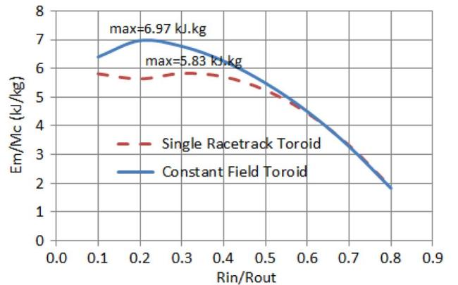
Fig. 6. Specific energy versus  $R_{in}/R_{out}$ .
