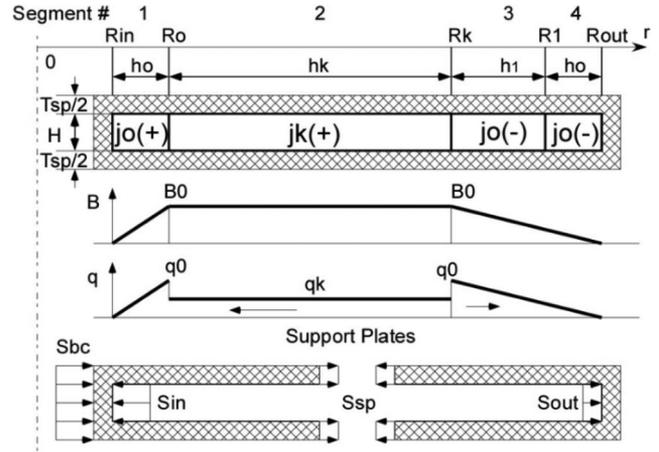
Fig. 8. Sizing TF coil support plates.
