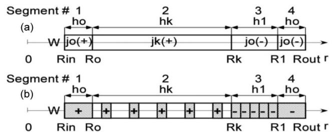
Fig. 2. Coil cross section (a) without and (b) with discretization.
