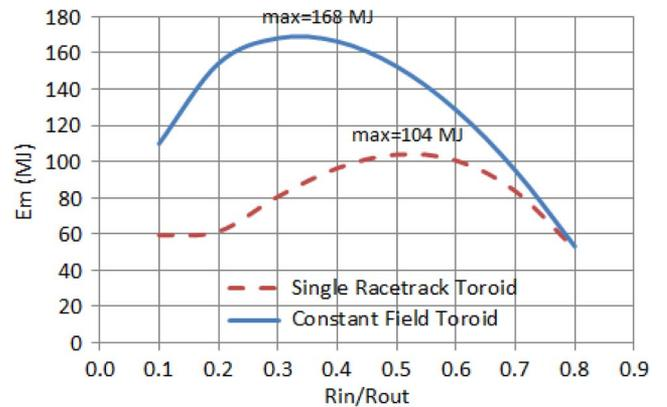
Fig. 5. Stored energy versus  $R_{in}/R_{out}$ .
