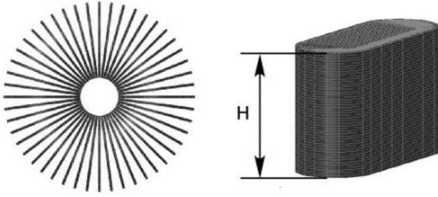
Fig. 7. Rearranging CFT coils into a stack.
