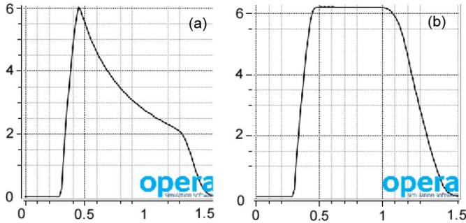
Fig. 3.  $B$  (in teslas) versus radius (in meters) at midplane in (a) SRT and (b) CFT magnets.
