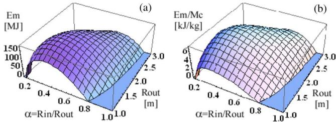
Fig. 9. (a) Stored energy  $Em$  and (b) specific energy  $Em/Mc$  versus  $(R_{out}, \alpha)$ , for  $V_{env} = 27 \text{ m}^3$ .
