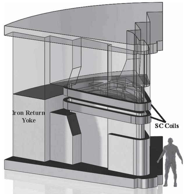
Fig. 1. Schematic of one sector of SRC showing two SC coils and the iron return yoke. The top half of the iron return yoke is transparent.
