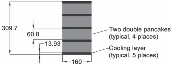
Fig. 2. Winding pack cross-section envelope consisting of four sets of two double (aka, quadro) pancakes sandwiched by five cooling layers. Dimensions are in mm.
