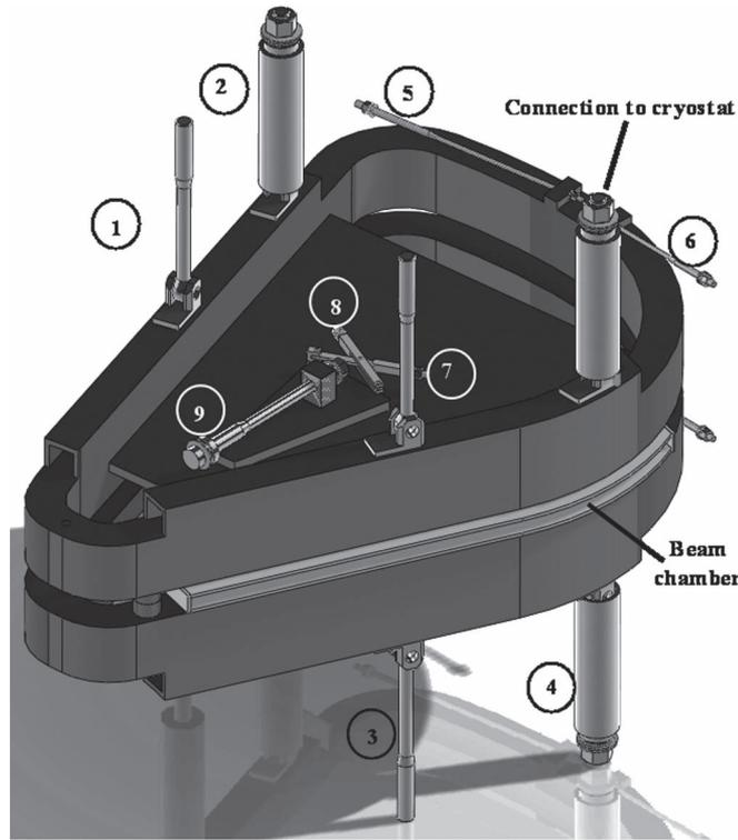
Fig. 3. Coil cases surrounding SC coils with numbered warm-to-cold support links. Supports #4 and #9 shown connection to cryostat.
