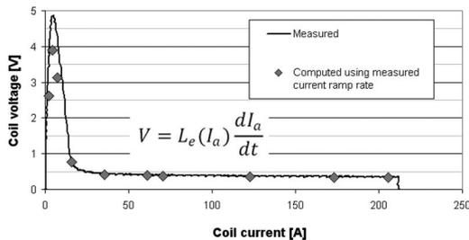
Fig. 4. Voltage across coil terminals versus current.
