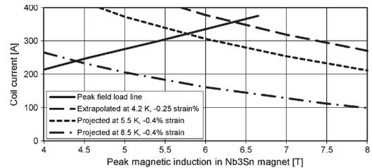
Fig. 2. Projected coil performance.
