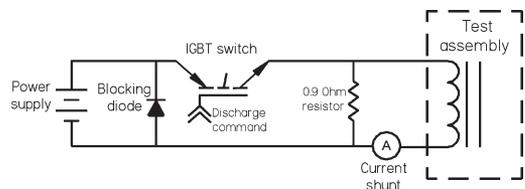
Fig. 3. Charging circuit schematic.
