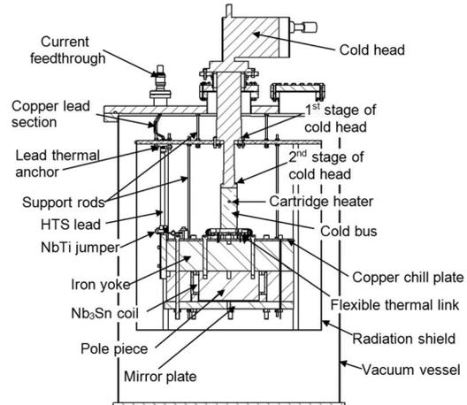
Fig. 1. Cross-section view of the test apparatus.
