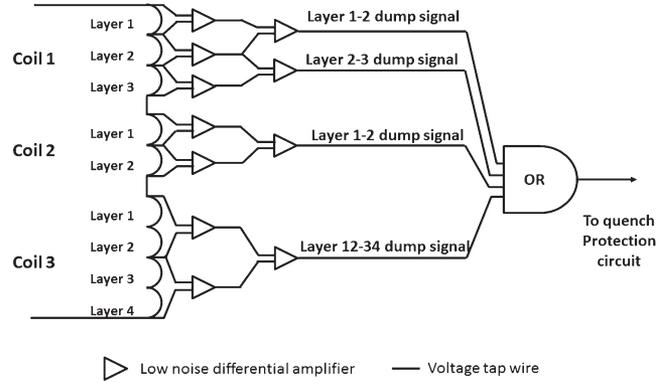
Fig. 4. Schematic of possible arrangement for voltage taps and signal processing. Wire twisting, isolation resistors, and tap redundancy are not shown.
