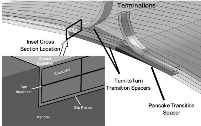
Fig. 3. Coil 2 pancake winding and layer winding along mandrel shown (mandrel is hidden). Pancake winding is transparent to display the spacers used for the pancake and turn-to-turn transitions. Inset indicates stack-up of slip plane, insulation and conductor on mandrel (mandrel is visible).
