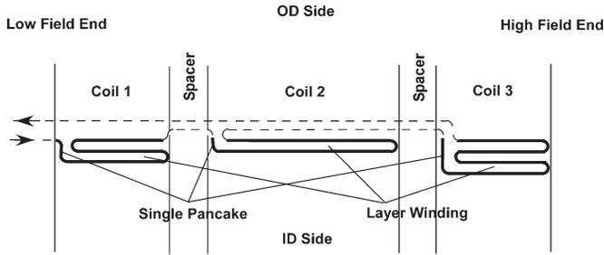
Fig. 2. Schematic of winding scheme showing each coil winding initiated with a single pancake and continuing with layer winding.
