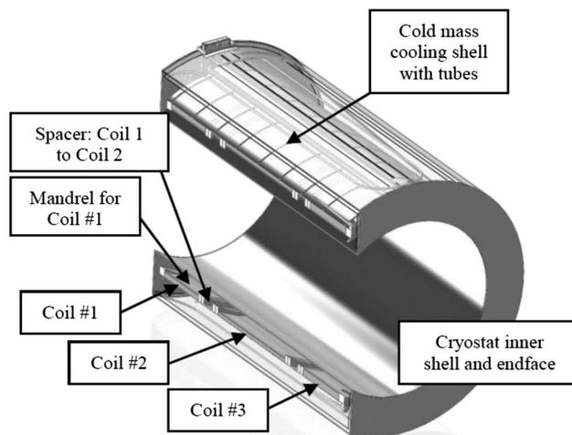
Fig. 1. Section view of the solenoid. Outer shell of both cryostat and radiation shield are transparent to view cooling shell.
