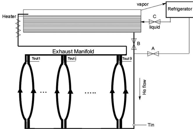
Fig. 5. Principal scheme of the magnet siphon cooling circuit. Pairs of arcs shown represent three of nine pairs of tubes carrying parallel He flow around cold mass OD. A, B, and C are valves and locations of temperature measurements are shown.
