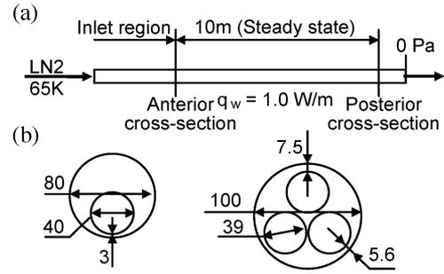
Fig. 3. Models of the geometries of pipe. (a) The parameters of the calculations along LN2 channel. (b) The hydraulic cross-sections of a single cable and three cables.
