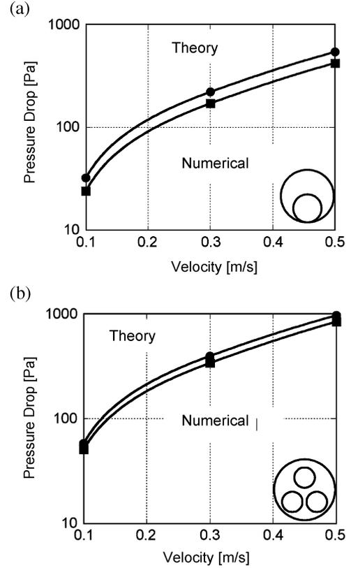
Fig. 5. Comparisons of the analytical results with theoretical results on fluid velocity dependence of the pressure drop. (a) For the single phase DC-SC cable. (b) For the three phase AC-SC cable.
