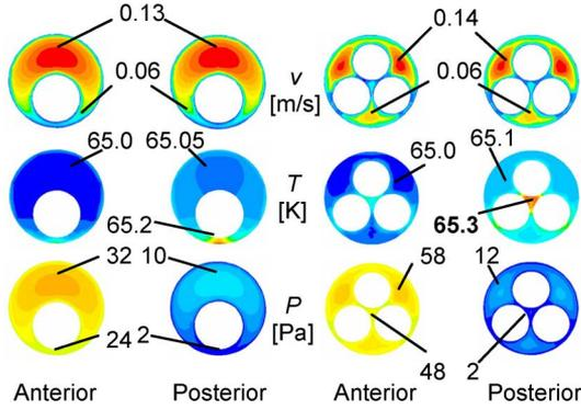
Fig. 4. The distributions of the fluid velocity, temperature and pressure at the anterior cross-sections and posterior cross-sections for the DC-SC and AC-SC cables.
