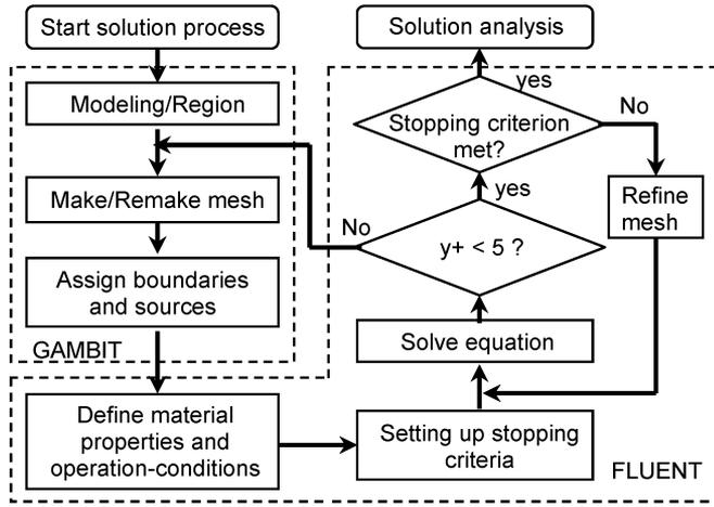
Fig. 2. Flow chart of the fluid analysis for the DCSC-PT system.
