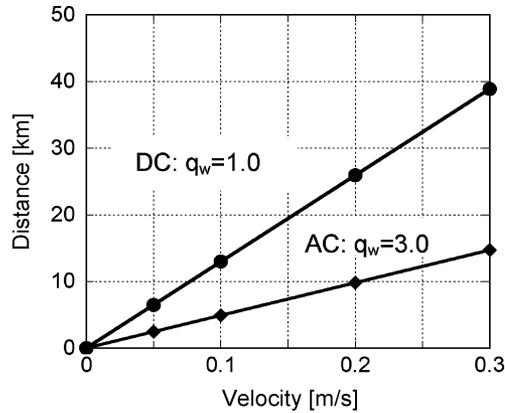
Fig. 6. The velocity dependence of distance between cooling stations. The distance for a DC-SC system is twice longer than that for a AC-SC system.
