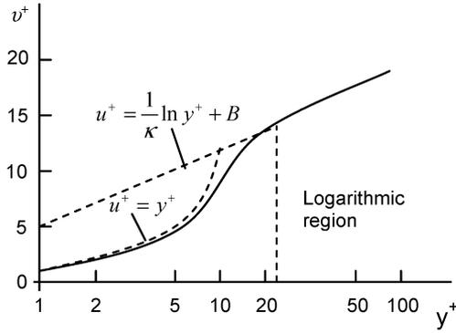
Fig. 1. The velocity profile of turbulence boundary layer as a function of distance normal to wall (dashed lines are from corresponding equations, solid line represents experimental data).
