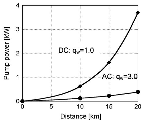
Fig. 7. The distance dependence of pump power to circulate LN2. When the cooling station interval is 10 km, the pump powers of a DC-SC PTL and AC-SC PTL are 0.13 kW and 0.63 kW, respectively. When the distance between cooling stations are 20 km, the pump power for the DC systems is one order lower than that of the AC systems.
