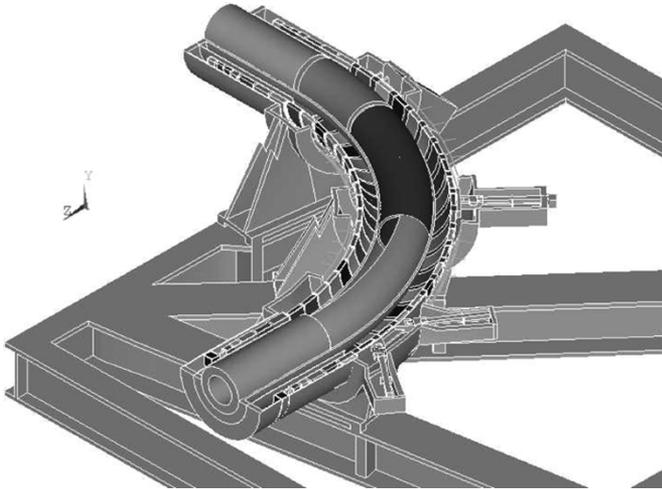
Fig. 4. Global TS model with shields. The upper half of the magnets and cryostat shells are shown removed.
