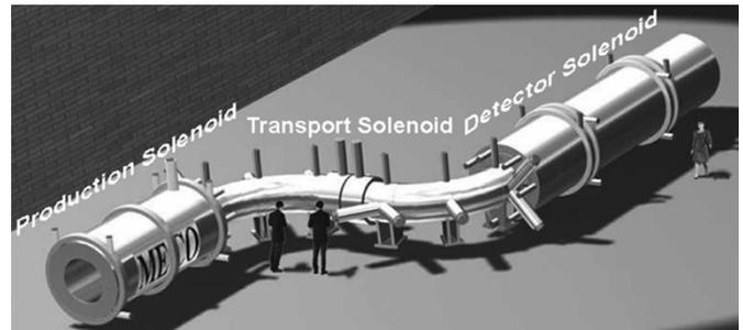
Fig. 1. MECO magnet system. Iron boxes around PS and DS removed.
