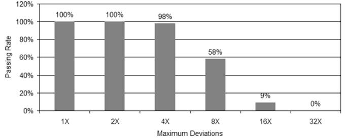
Fig. 3. Field spec passing rate for the cumulative errors due to machining tolerances on dimensions of outer mandrel surfaces.
