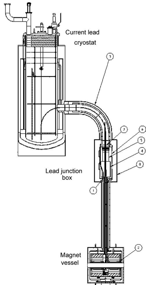
Fig. 3. Section view of cryostat to measure heat load on the prototype HCX quadrupole doublet beam focusing magnet.
