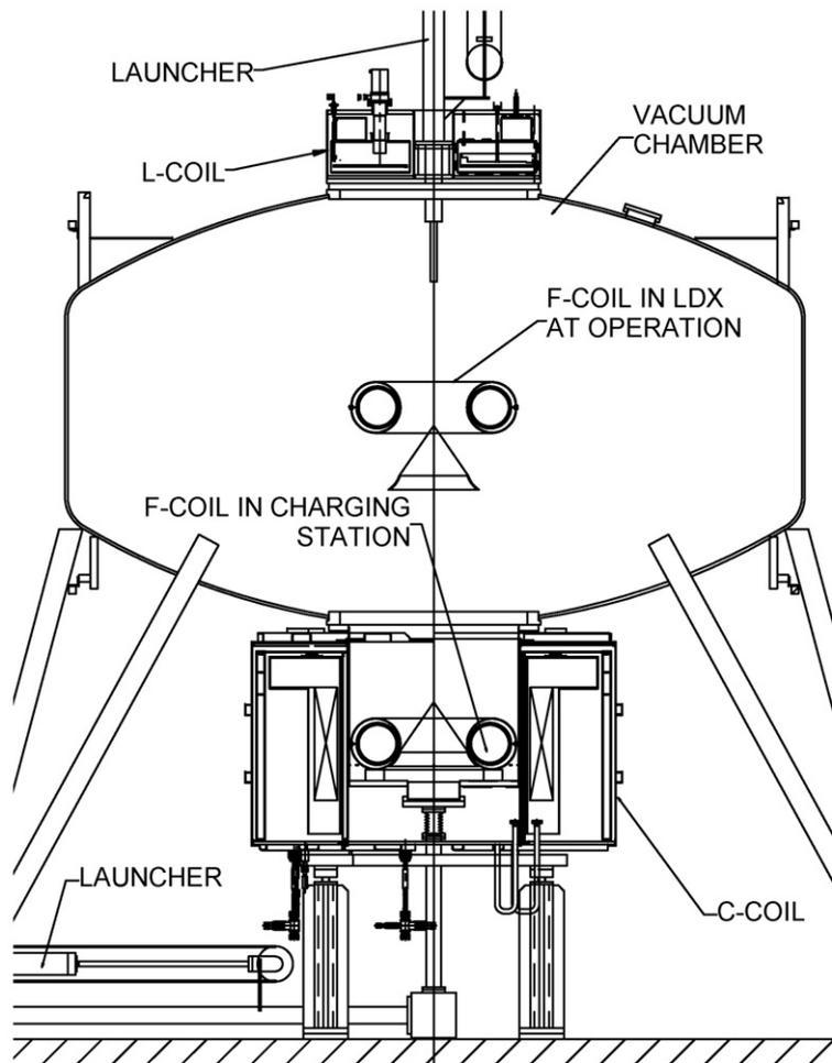
Fig. 4. Section view of LDX showing relative locations of the superconducting magnet systems.
