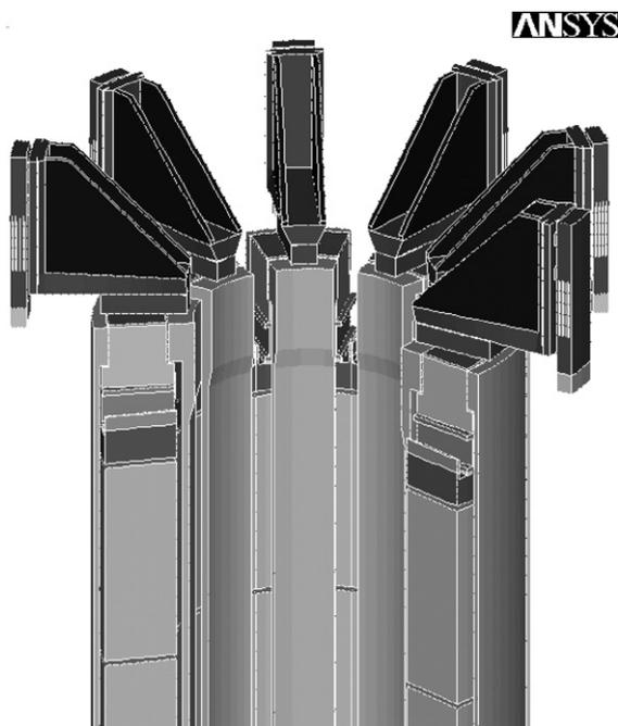
Fig. 2. Coarse mesh, 360° ANSYS model for the ITER CS with upper mounting structure.
