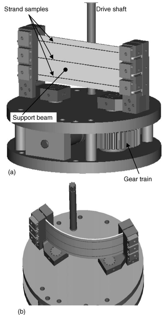
Fig. 1. Variable bending, strand test apparatus at (a) zero bending and (b) constant radius of curvature test positions.
