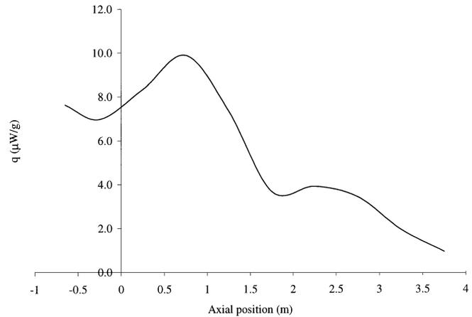
Fig. 2. Azimuthal peak nuclear heating in the PS vs. axial position. The field specification region begins at  $z = 0$ ; the PS winding begins at  $z = -1$ .
