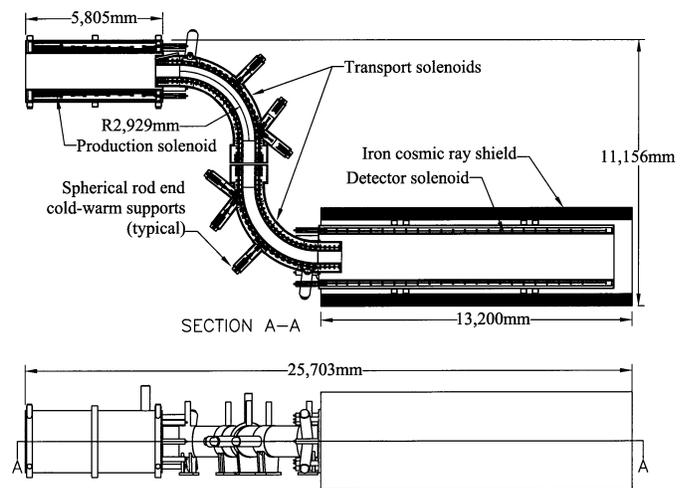
Fig. 1. Layout of the MECO solenoids.
