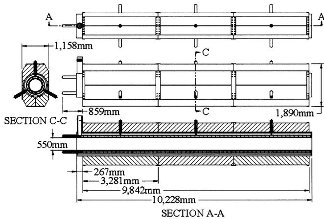
Fig. 1. Elevation, plan, and cross-section views of the Case II coil, cryostat, structure, and iron yoke.
