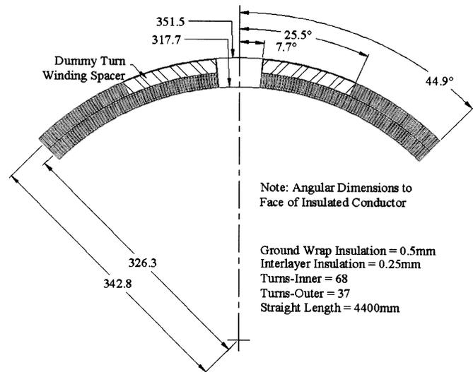
Fig. 3. Elevation, cross-section view of two layer winding and pole piece.
