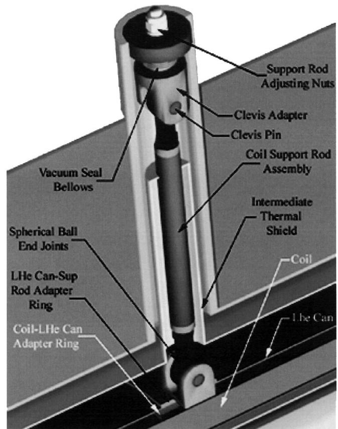
Fig. 5. Cold-warm gravity support rod assembly.
