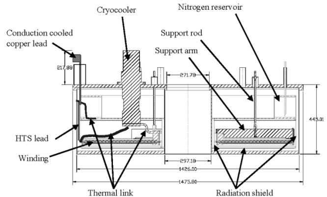
Fig. 1. Section view of the L-coil winding and cryostat.
