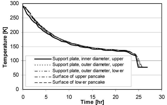
Fig. 4. Temperature vs. time traces during conduction cooling of the L-coil.
