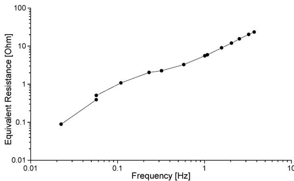
Fig. 6. Equivalent a.c. loss resistance for the L-coil vs. excitation frequency.
