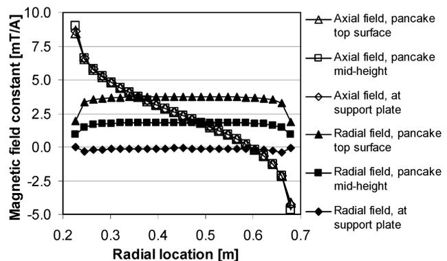
Fig. 2. Variation in the axial and radial magnetic field constants vs. radial location, at three vertical heights in the L-coil upper pancake.
