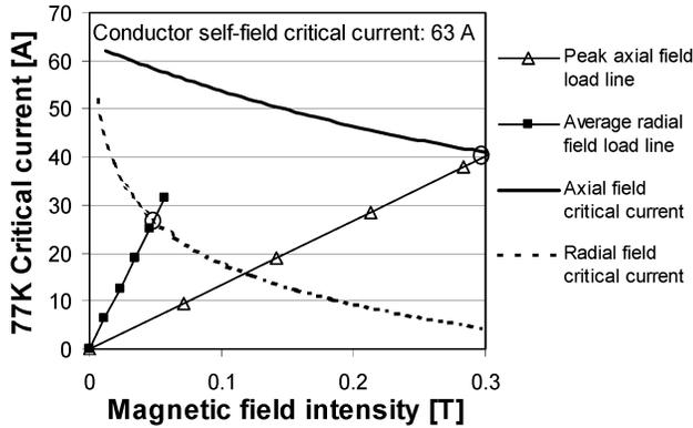
Fig. 3. 77 K critical current vs. background field intensity for L-coil conductor exposed to axial and radial magnetic fields. Load lines for the coil's peak axial field and the average radial field at the mid-height of the pancakes are over-plotted in the figure. The L-coil critical current (28 A) is determined by the lower intersection of load line and critical current curves.
