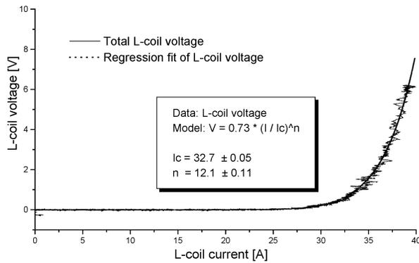
Fig. 5. L-coil voltage vs. current trace during a critical current measurement using a 0.04 A/s current ramp to 38 A.
