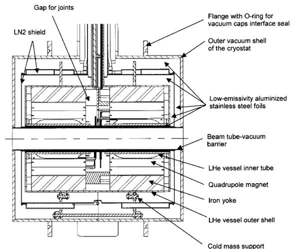
Fig. 5. HCX prototype cryostat.
