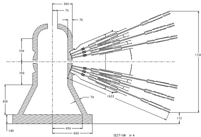
Fig. 6. Final focus triplets (6 beam lines) and HIF reaction chamber. (dimensions in cm).
