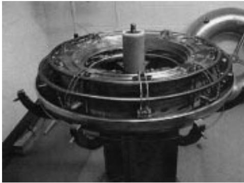
Fig. 5. The lower half-vessel installed in the cryostat assembly apparatus. The upper half-vessel is seen behind. The magnet with the heat exchanger is installed in the lower half-vessel.
