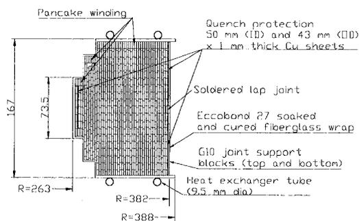
Fig. 1. Floating coil winding (dimensions in mm) is contoured to fit into a toroidal shell. Heat exchanger tubes for recooling are also shown. Finished coil has about 720 turns.
