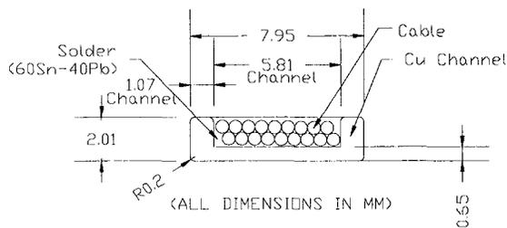
Fig. 2. Floating coil conductor cross section
