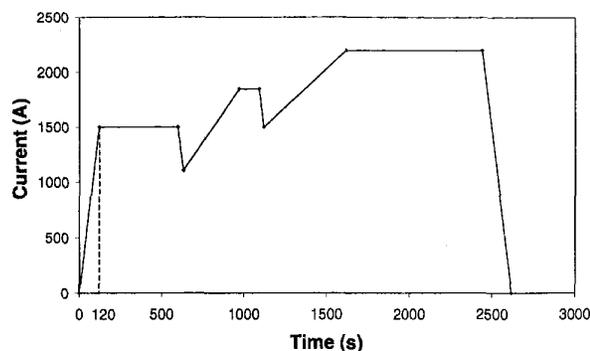
Fig. 6. First current ramp sequence of the floating coil to 2200 A or 106% of full planned operating current. Additional ramps were made, also. The coil never quenched.
