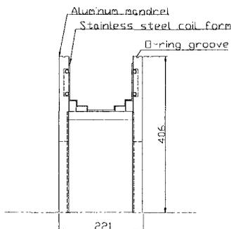
Fig. 3. Coil form in winding mandrel (upper half only)
