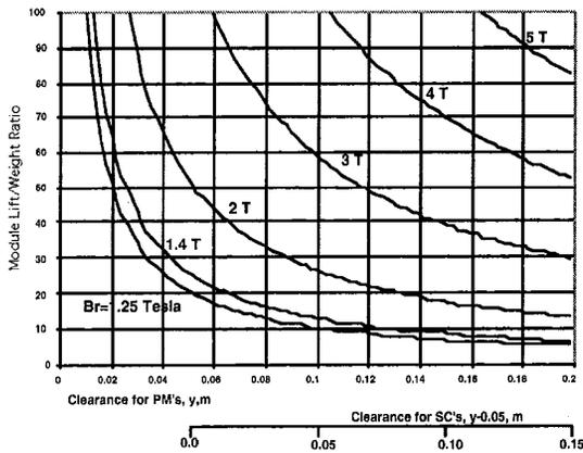
Fig. 6. Approximate lift to weight ratios vs clearance to the guideway for permanent magnets and superconducting coils. Halbach array used for PM or for wound SC coils. PM is limited to  $Br < 1.4$  T.
