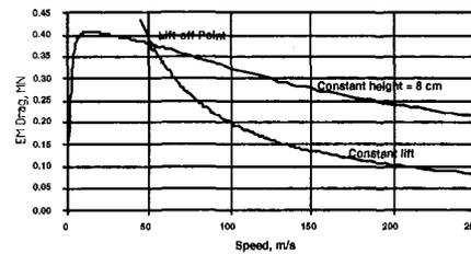
Fig. 3. EM drag due to interaction of 4 levitation modules with a 2 cm Al guideway for a constant height before lift off and constant lift of 590 tonnes after lift off.
