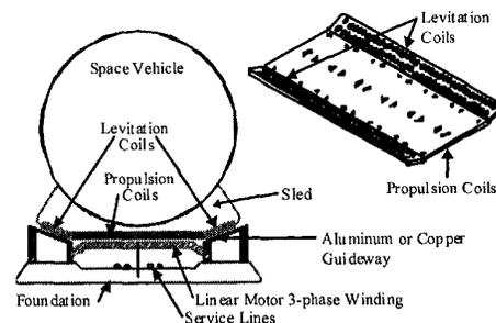
Fig. 1. Cross-section of vehicle, sled, bogie and guideway, with an isometric of the coils in one bogie.
