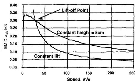
Fig. 5. Electromagnetic drag for a 590 tonne vehicle due to the interaction of the levitation coils ( $2.9 \times 10^5$  At per coil) with a 2 cm Cu guideway.
