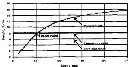
Fig. 2. Height, H, for the levitation module cryostat relative to the guideway vs speed for a 590 tonne vehicle, a 2 cm Al guideway and  $3.2 \times 10^5$  ampere turns per lift coil. Clearance is (H-6 cm).
