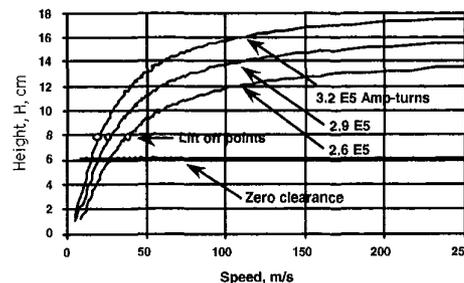
Fig. 4. Height, H, for the levitation module cryostat relative to the guideway vs speed for a 2 cm Cu guideway and selected lift coil ampere turn levels for a constant lift of 590 tonnes. Clearance is (H-6 cm).
