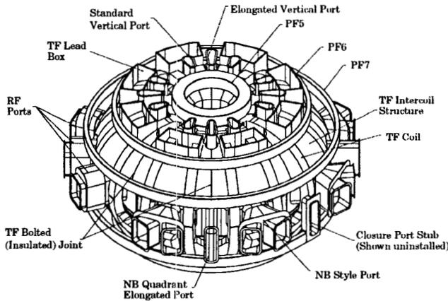
Figure 1: KSTAR general arrangement with magnet system
