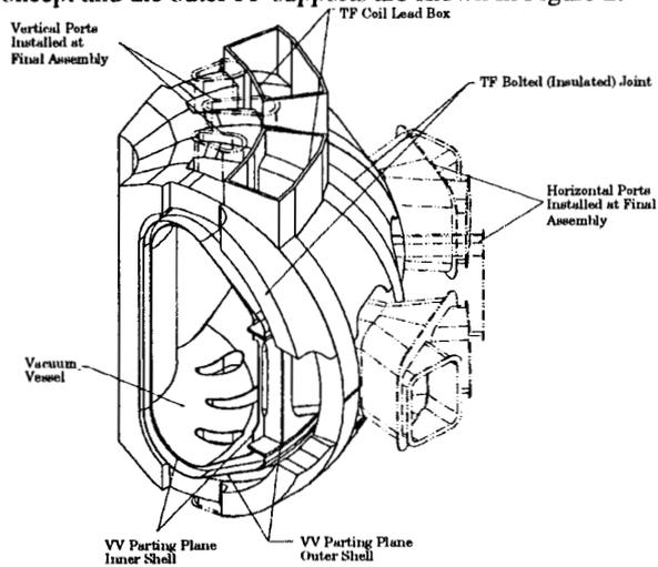
Figure 2: TF Coil Quadrant Assembly with PF Supports
