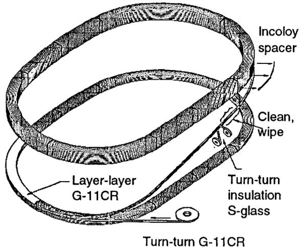
Figure 3: Insulation of Continuous Wound TF Coil
