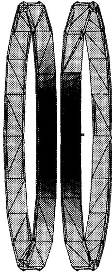
Fig. 2. Heat flux into the winding pack. Darkest region shows the location of the peak heat flux of  $25 \text{ W/m}^2$ .
