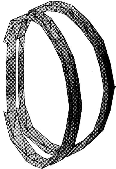
Fig. 3. Heat Flux into Case Cooling Channels. Darkest region represents a heat flux of about  $300 \text{ W/m}^2$ .
