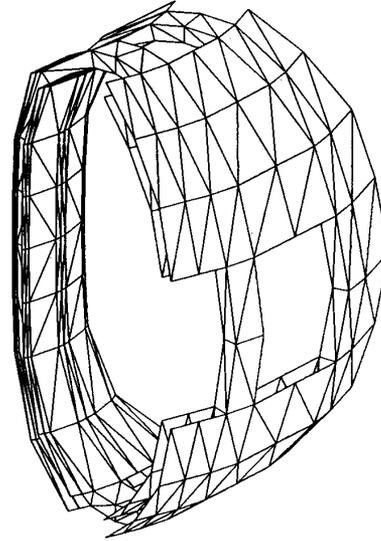
Fig. 1. Isometric view of 3-D thermal model, two TF coil subassembly.
