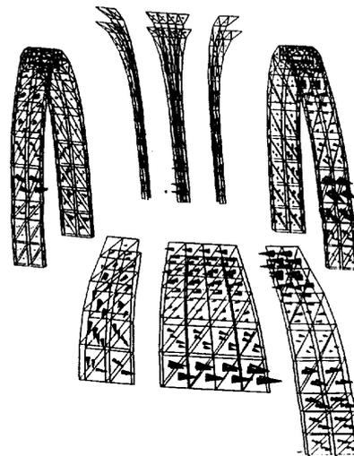
Fig. 10 Eddy Currents in the Structural Elements of the TFCCS
