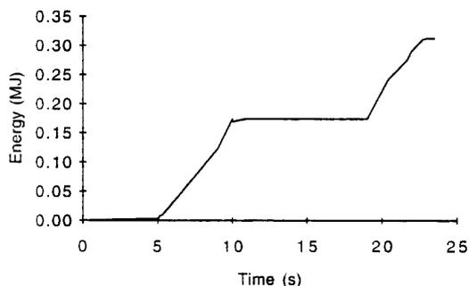
Fig. 7 Energy of Joule Heating of the TF Cold Structure
