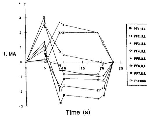
Fig. 5 Currents in the PF Coils
