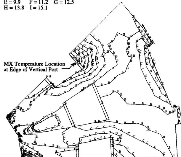
Fig. 11 Temperature Contours in TF Coil Case Structure at 23s
