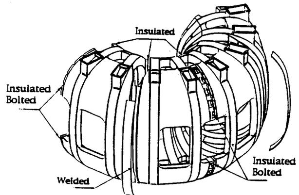
Fig. 2 TPX TF Coil Cold Structure (TFCCS)
