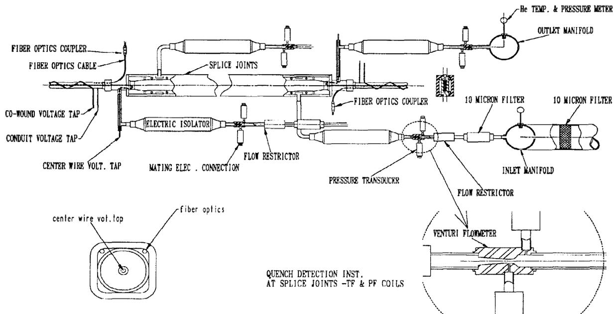
Figure 5: Quench Detection Sensor Concept for TPX
