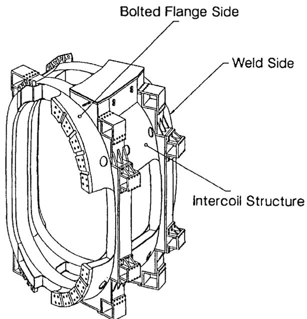
Figure 2: Two TF Coil Assembly with Outer PF Supports
