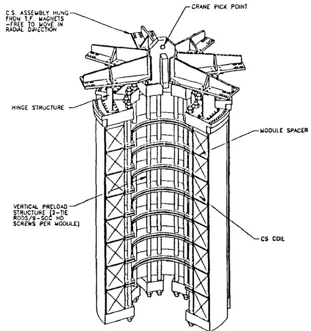
Figure 4: Central Solenoid Assembly
