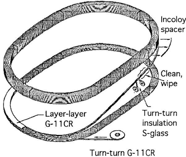
Figure 3: Insulation of Continuous Wound TF Coil
