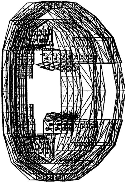
Fig. 6 Eddy Currents in the Structural Components
