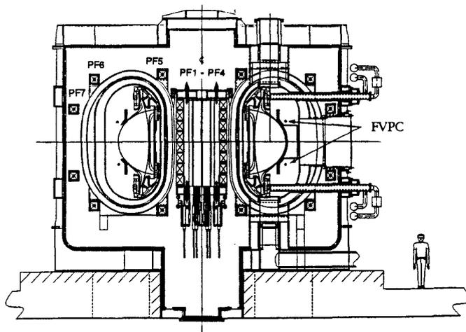
Fig. 1 TPX Elevation View
