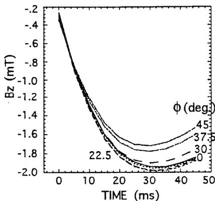
Fig. 11 Bz at R=2.5 m at Different Toroidal Positions as a Function of Time
