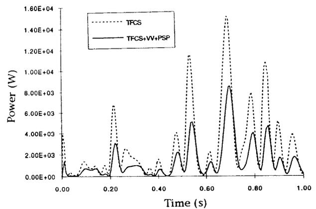
Fig. 5 Power Dissipation in the TF Cold Structure
