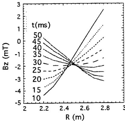
Fig. 10 Bz versus Radial Position - 3-D Calculations
